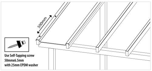
Fix the first SUNTUF EZ Glaze panel's outer corrugation, using specified screws and washers through the pre-drilled holes. Start at the bottom edge and work your way up.
